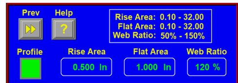
**Rise Area** – The distance the label travels before changing to the flat area speed. The applicator will run at web speed during rise area.
