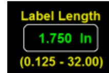
To change a value the operator will touch the screen inside the box and a keypad will appear on the screen. As numbers are inputted into the keypad the value will change. Pressing “ENT” will close the keypad and confirm the change. Pressing “ES” will close the keypad and cancel the change. Pressing “CR” will clear the inputted value. If the operator presses “ENT” after inputting a value outside of the limits the value will revert to its’ original value.
