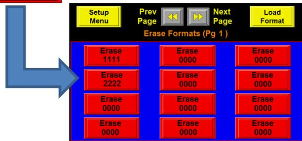
When the operator selects a format to erase will remove the format name to show “0000” instead. There is no second step and formats cannot be retrieved once erased.
