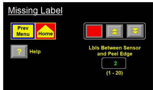
**Labels Between Sensor and Peel Edge** – The number of labels from the label sensor (counting any label currently under it) to the peel edge (counting any label hanging past the edge).
