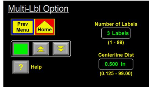
**Number of Labels** – The number of labels, including the original apply, that the applicator will apply based off a single product detect.
