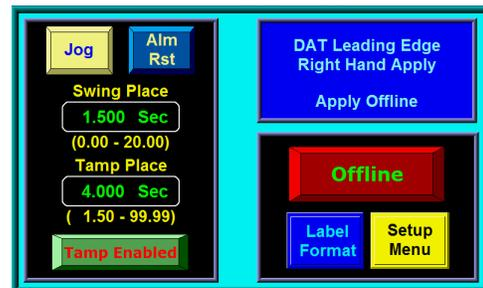
**NOTE:** If the first part of the cycle is not completed by the time / distance of the second label placement has passed the second label will be applied late and a warning alarm will be generated. To correct, shorten the cycle time of the first cycle or decrease product speed.
