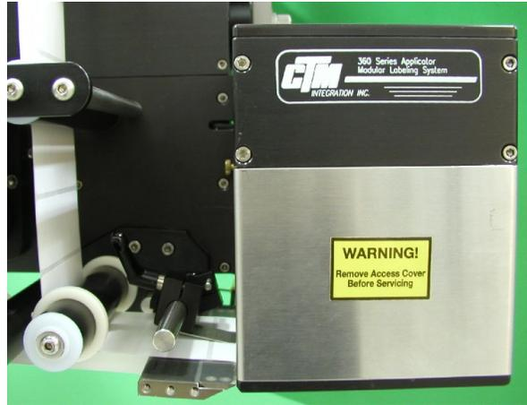
1. Under applicator type in the configuration menu of the display, select “air blow” applicator. Also, indicate whether it is in a right-hand or left-hand configuration. If there were any options turned on, they will be turned off when changing applicator types. If the dispense direction is changed and the applicator type menu is exited, the applicator will force the operator to cycle the power to the applicator before any other changes can be made.
