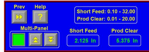
**Short Feed** – The distance the label is fed after label placement on product detect. This move is done at encoder speed. This will be taught by doing an auto teach of the label sensor with the multi-panel option enabled.
