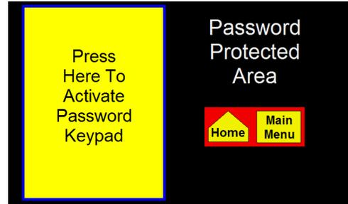
Once the password has been entered you may hit “ENTER” to confirm it. If entered correctly you will advance to your desired screen. If an incorrect password is entered a screen will be shown to notify the operator. In the even that you know you have hit the wrong number pressing “C” will clear the current entry.
