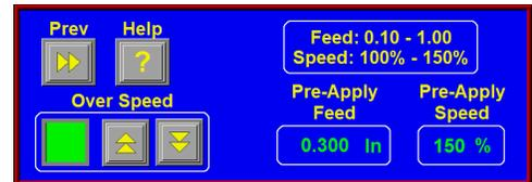
**Pre-Apply Feed** – The distance that the applicator will feed at the higher speed while over speed is turned on.
